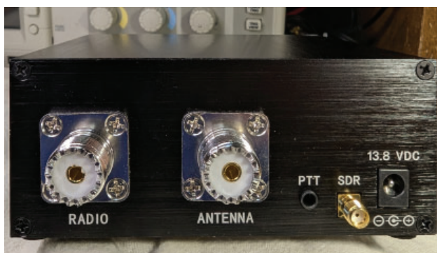
Figure 9 — Rear of the SDR TX/RX switch.
