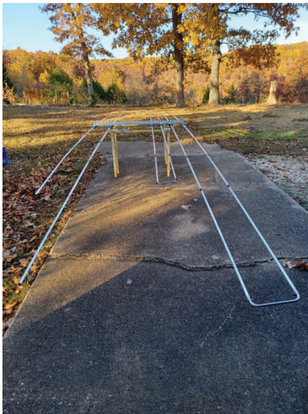
Figure 5 — The 1712DUO elements and boom assembled prior to adding the boom-to-mast plate and plastic element stabilization strips.
