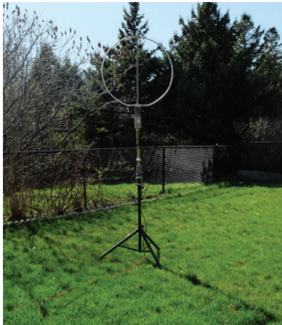
Figure 16 — The PWRC setup with a low-noise loop.
