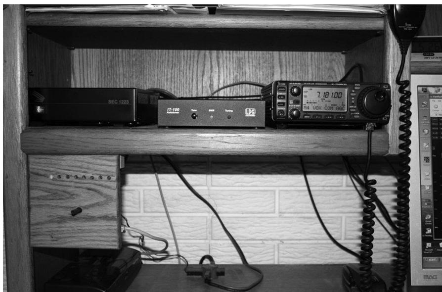
Figure 2 — This photo of my operating position shows my power supply, LDG Autotuner, and Icom IC-706 MKIIIG radio. The antenna selector control panel is mounted behind a block of wood to match the operating position shelf. You can see the selector shaft, with the first of eight LEDs illuminated to show which antenna has been selected. I still have to add labels below the LEDs to help identify the antennas.
