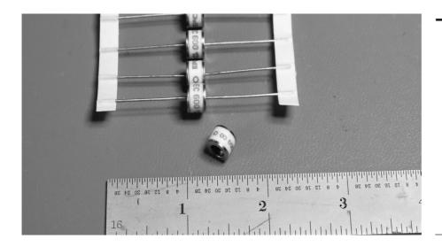
←Figure 2(a) — Axial lead format of EPCOS discharge tube.
