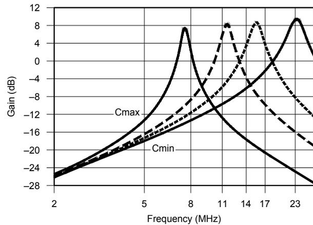
Figure 3 — Four frequency response curves of the tuned preamplifier as capacitor  $C$  is varied.
