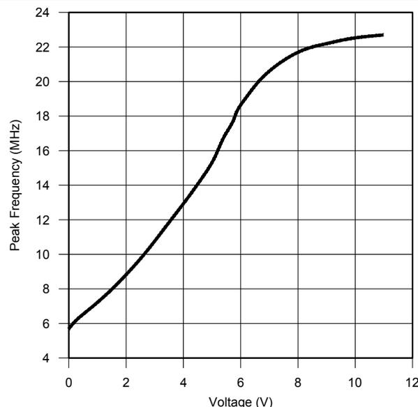
Figure 5 — Variation of peak frequency with varicap voltage. Data is taken for the 1SV149 used in the project. Frequency range is about 6 to 23 MHz.
