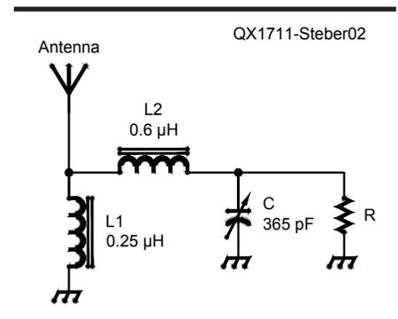
**Figure 2 — Classic tunable RF band-pass filter with variable capacitor *C*. Resistor *R* represents input to next stage, usually a FET amplifier.**
