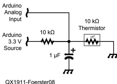
Figure 8 — Thermistor circuit.
