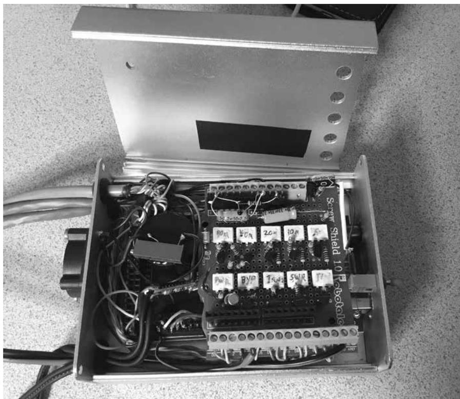
Figure 7 — Internal view of the Arduino housing.
