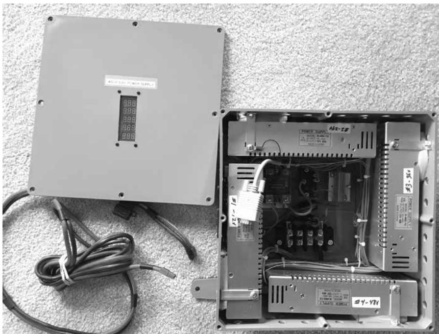
Figure 5 — Layout of the power supply.
