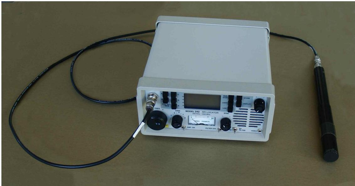
**Figure 65 Radar Engineers Noise Receiver with Probe**
