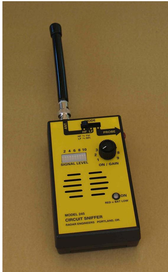
**Figure 67** Circuit Sniffer Used to Locate On-Site Sources
