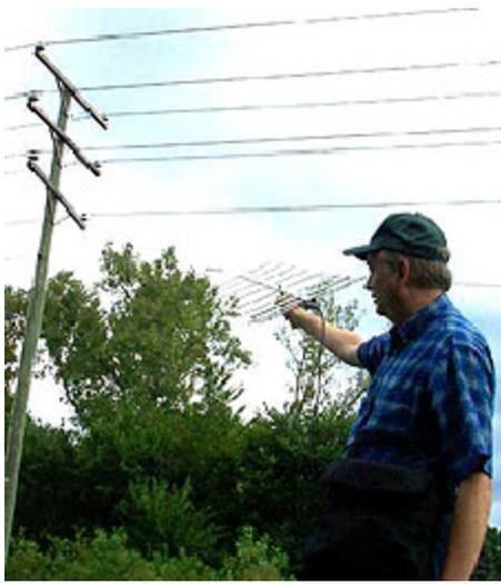
ARRL EMC Engineer Mike Gruber, W1MG, demonstrates one technique for pinpointing power line noise.
