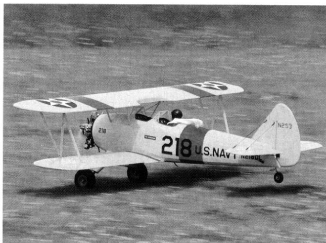
Don Forte's big PT-17 scale model is on its take-off roll. The model spans 78 inches and has a five-cylinder rotary engine. (The original PT-17s had nine-cylinder engines.) This World War II trainer model can perform stunts that the full-scale original cannot. It's shown here in US Navy colors.
