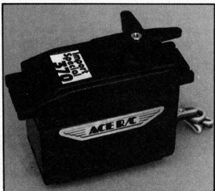
This Ace R/C model 370 servo is the "giant" in the company's lineup. The splined shaft (top right) rotates up to 90° (the four-pronged output arm mounted on the shaft allows for mounting and installation flexibility). The tabs on the "skinny sides" are for mounting the device. (photo courtesy of Ace R/C, Inc)
