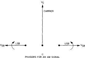
PHASORS FOR AN AM SIGNAL AT ARBITRARY INSTANT REFERENCED TO CARRIER
