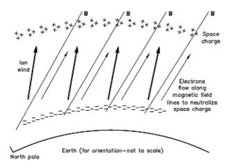
Figure 4—At mid-latitudes, electrons flowing along sloping magnetic field lines B quickly neutralize any charge above or below the ionosphere created by a vertical electric current.
