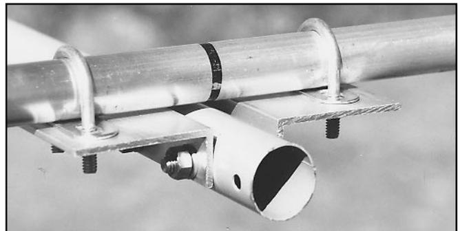
**Figure 1**—Two pieces of angle aluminum are attached to the boom with two nuts, bolts and lock washers. Your drilling must be accurate, so use a drill press if possible. In addition to drilling the boom holes, you'll need to drill four holes in each angle piece: two for accepting the boom-mounting nuts and two for the U bolts that will hold the element.
