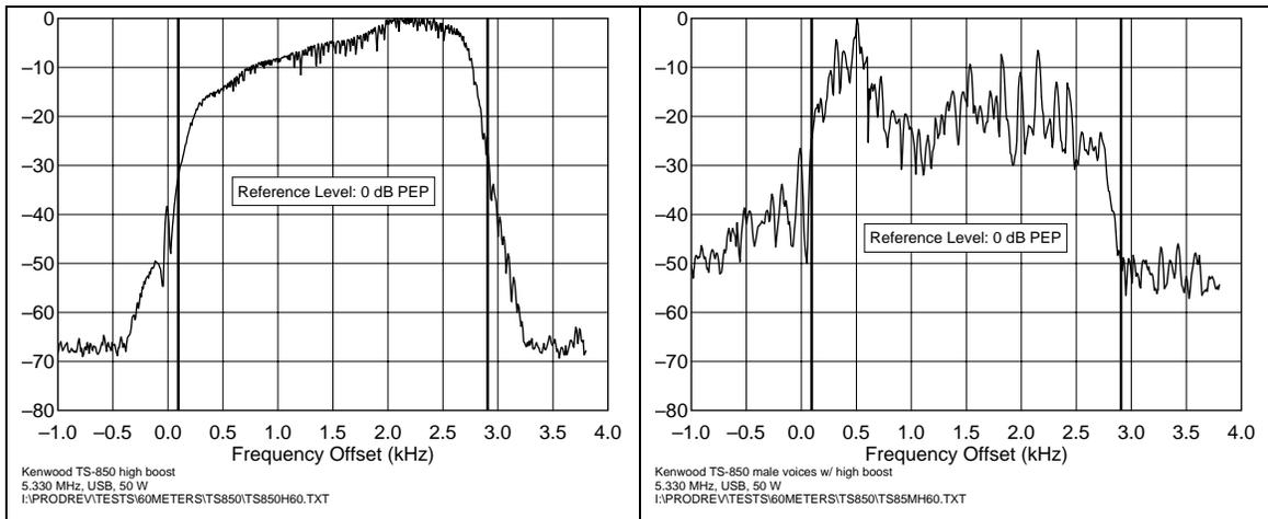
On the Kenwood TS-950 (an unmodified transceiver), several tests were performed on 3.9 MHz in USB (so as to match the filter shape that would be observed on 5.3 MHz). The first plot of this group is the swept audio response of the transceiver. The second plot is the response to voice input (both male and female voices were used for this test). The third plot is the response of a male voice with the processor enabled.
