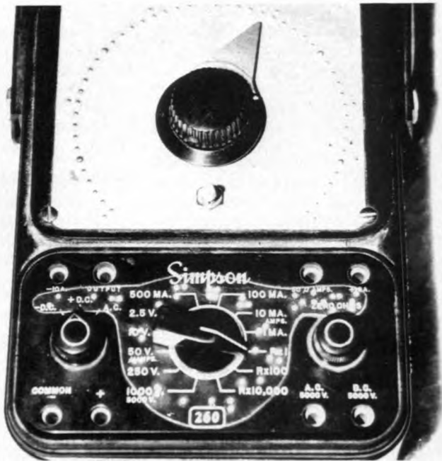
Fig 2—A Simpson 260 VOM outfitted with a Braille dial and a tone generator. The pointer-equipped knob is turned until the tone is nulled out; then you read the Braille scale. Since this is a linear scale, a Braille conversion table must be used for reading resistance.
