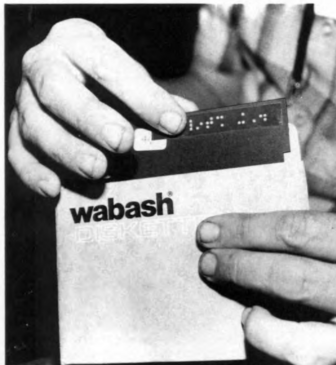
Fig 1—Here's how the Dymo label is used to identify a floppy disk. (photos by Gary McDuffie, AG0N)
