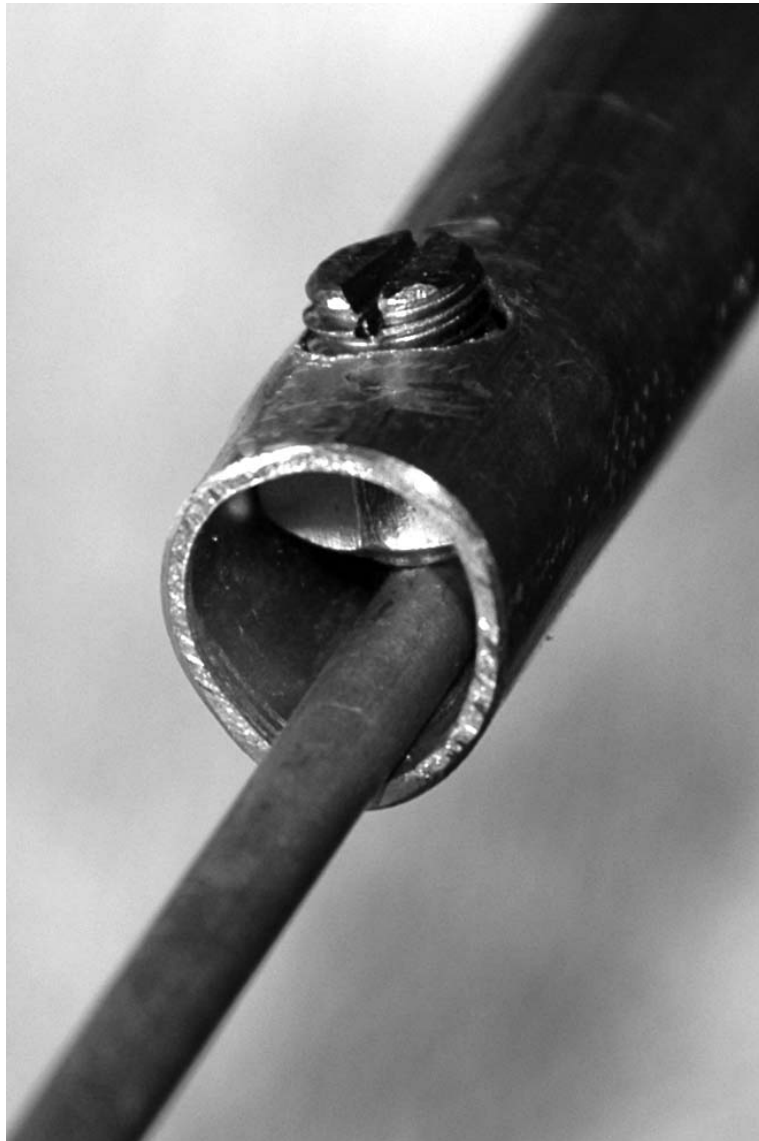
Figure 5 — A close-up view of the anchored end of the linear resonator tube. Note the positioning of the modified bolt and nut used to fasten the rod in place.
