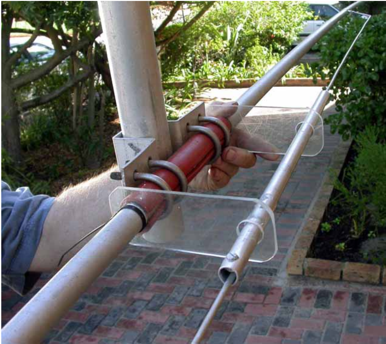
Figure 2 — The 15 meter linear resonator assembled onto the 20 meter reflector.
