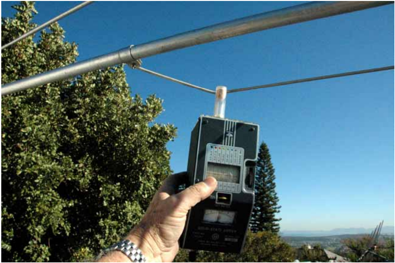
Figure 8 — Using an absorption dip meter to bring the linear resonator to proper resonance.
