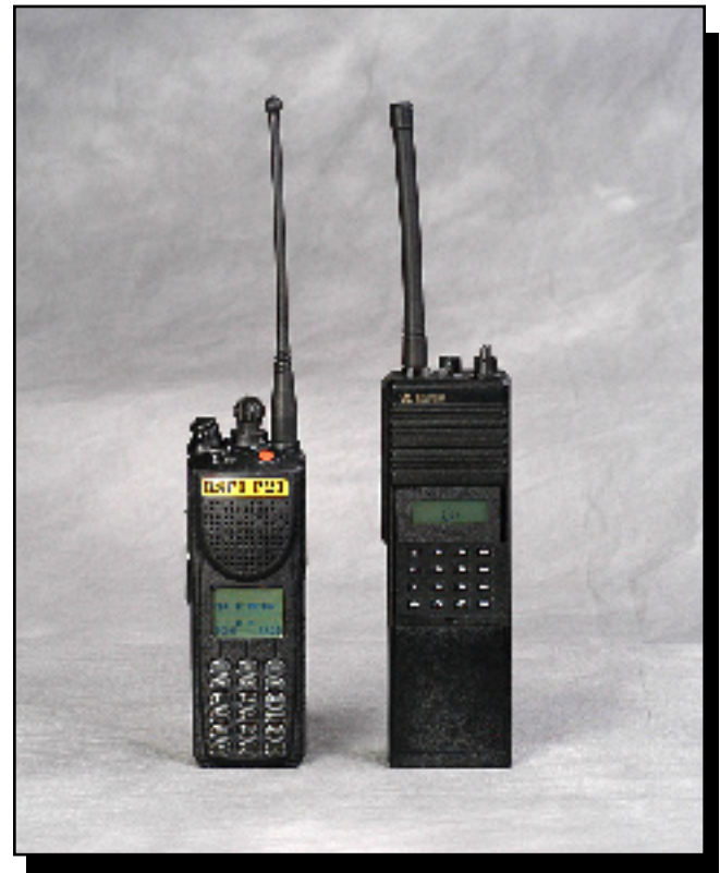
Figure 1—The newer UHF Motorola Astro XTS 3000 radio (left) and the VHF Bendix-King radio. Both radios have “rubber duck” antennas.
