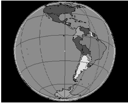
Figure 1—The Earth as seen from OSCAR 13 (as depicted by InstantTrack satellite-tracking software). In this view, the satellite is centered over the Pacific southwest of Peru. When OSCAR 13 was in this position, nearly every satellite-active ham in the continental US could work stations throughout the Caribbean, Central America, South America and a large portion of the South Pacific.
