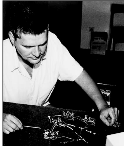
Matjas Vidmar, S53MV, is shown experimenting with prototypes of the LEILA circuit for the Phase 3-D satellite at his workshop in Slovenia. It is designed to alert ground station operators who inadvertently run too much uplink power by superimposing a warning message on the "offending" station's downlink signal.
