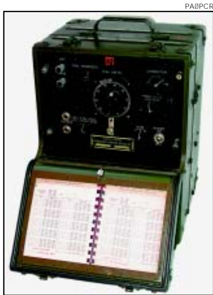
Figure 4—The SCR-221/BC-221 frequency meter, a precision instrument used in both military and civilian applications.
